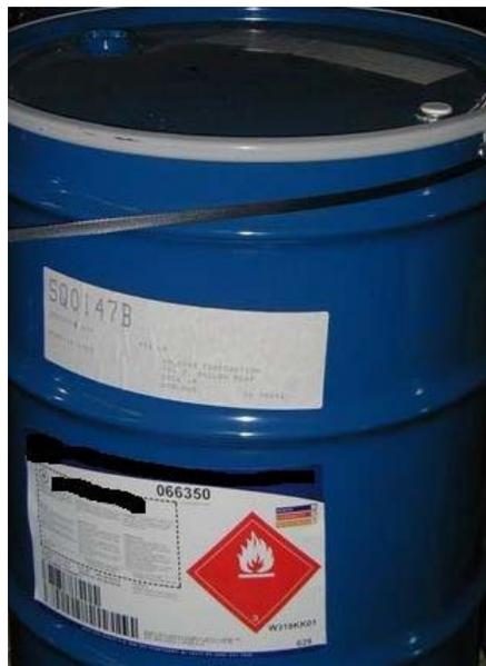
This drum is missing several fields of information and the bar codes for all the fields. This example **does not comply** with the requirements.
