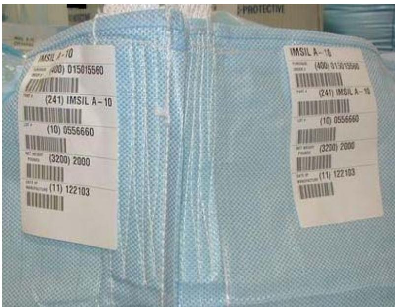
This Super sack has Valspar Bar Code Labels on adjacent sides of top portion of super sack. This example meets the requirements.
