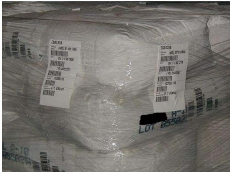
Each bag is labeled with a Valspar Bag Label on the side or end of the bag. The skid is shrink-wrapped and two Valspar Bar Code Labels are applied on adjacent top corners of the skid. This example meets the requirements in this document.
